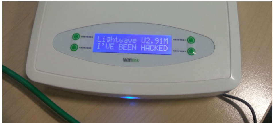
Figure 2. Smart hub device running modified firmware
