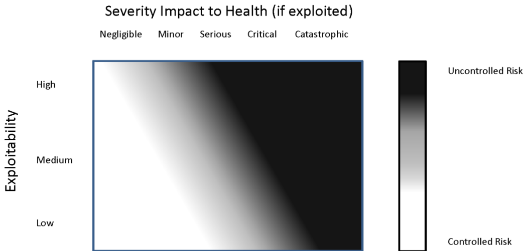
Figure – Evaluation of Risk to Essential Clinical Performance. The figure shows the relationship between exploitability and risk to health, and can be used to assess the risk to the device’s essential clinical performance from a cybersecurity vulnerability. The figure can be used to categorize the risk to essential clinical performance as controlled or uncontrolled.
