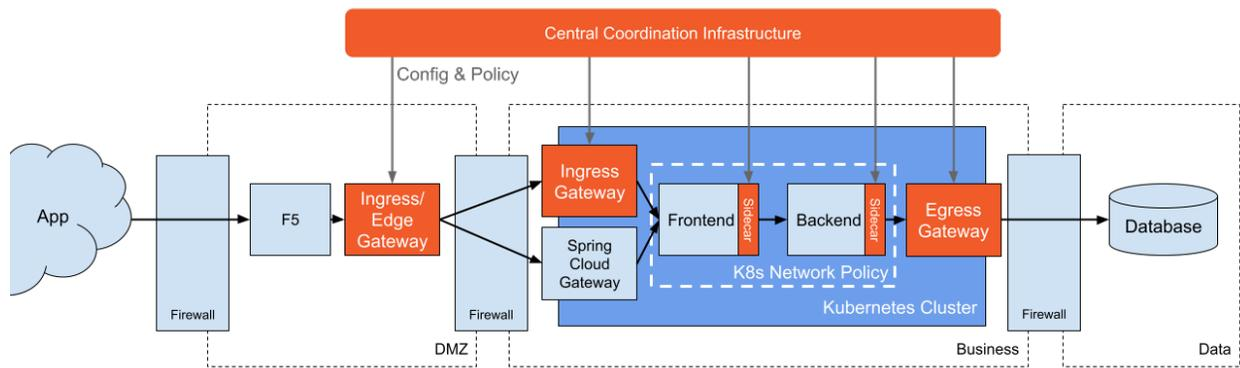
Fig. 5. Policy deployment for a three-tier application
